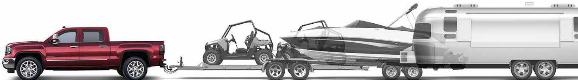
**TRAILER SWAY CONTROL** This technology helps keep both you and your trailer heading in the same direction, automatically. It detects a swaying trailer and applies both the vehicle's and the trailer's brakes (if properly equipped) to help bring it back in line.
